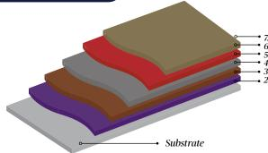
1. **SEE STAGE 1 - SURFACE PREPARATION EPOXY RESIN WITH MICROBALLOONS OR** 2. **EPOXY FILLER** Spot fill minor defects. SAND LIGHTLY DE-NIB.
