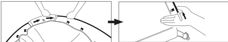
**IMPORTANT: DO NOT BEND THE POLE TO INSERT THE SECOND PIN.**
