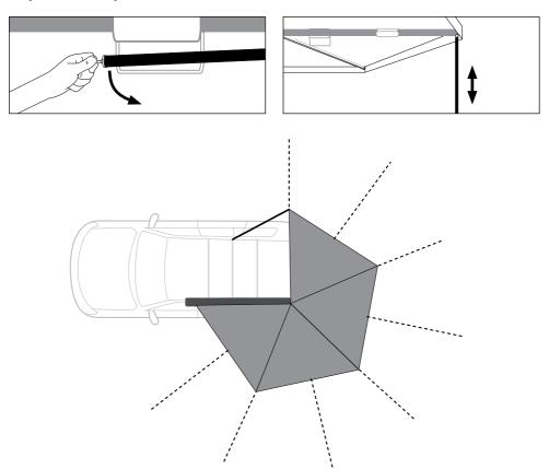
Undo the hook and loop fasteners that support each leg, taking care to support each leg as they pivot down to a vertical position. Adjust to the desired leg height by unlocking and locking the twist lock mechanism.
