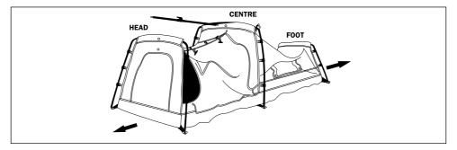
At this point you should have all three aluminium poles assembled, located in their corresponding positions and have centralized the swag at each point. The clips should all be attached to the aluminium poles on each side. Stretch out the base of the swag to ease assembly when placing the trigger lock spreader pole.
