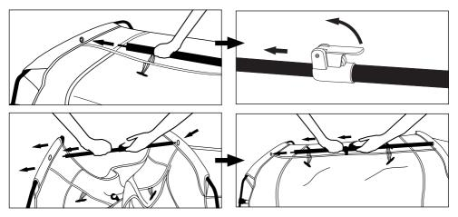
Insert the trigger lock spreader pole into the centre eyelet. Release the trigger to extend the pole and insert into the end eyelet. Tension the bar to stretch the swag into shape then lock into position and add the top clip. Peg out guy ropes at both ends, now your Outback swag set up is complete.
