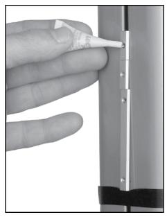
One drop blue Loctite® adhesive into each splice slug hole.
