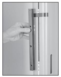
Slip top track slugs into mast groove. Use 32 mm  $(^{3}/_{4}")$  mounting slug for top stop.
