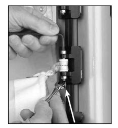
If screw extends below nut, it is overtightened.
