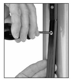
Hold full-length track piece up to mast. Loosely install top screw.
