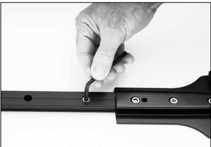
With track off mast, tap upper splice link into track using procedures outlined above.
