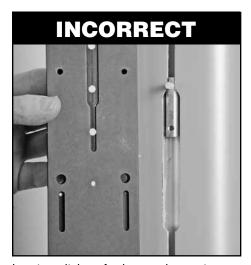
Locate switch so feeder gap does not interfere with mounting slugs.
