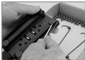
3. Remove retaining clips and corner keepers over box to catch balls.
