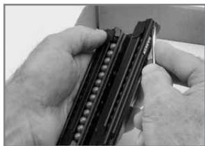
1. Use flat-bladed screwdriver to push retaining clip toward end.
