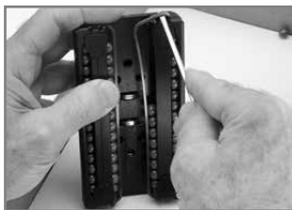
2. Pry retaining clip off and dump balls in box.
