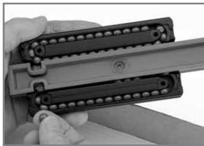
6. Put one (1) clip on "open" end of loader. Load rest of balls through ball loading port into empty bearing race. Consult chart to confirm quantity. Line up car loader with track and gently roll car onto track.
