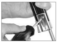
Coat screw with blue Loctite<sup>®</sup> and tighten. If screw does not thread, check alignment.
