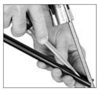
Cut, splay, and snap tube into place.
