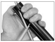
Splay foil with screwdriver and pull onto stay. Once foil is started, stop to install trim cap. *Tip:* Foil installs easier if excess is held out to starboard side of boat.
