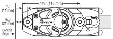
Drill  $^{27}\!/_{64''}$  (10.5 mm) hole through top surface of track only. Important: Do not use screw hole in control block as a drill guide.
