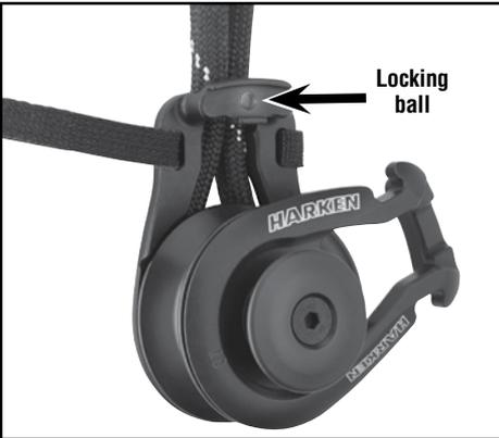
3. Rotate the cheeks to load line on sheave. Close cheeks making sure they align: there will be a clicking sound as the locking ball seats. The 3303 block has a pull pin, not a locking ball.
