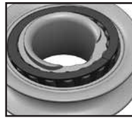
Split bearing cage and cutout in inner race lip
