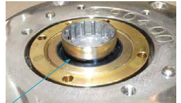
Lubrication of motor drive shaft lip seal.
