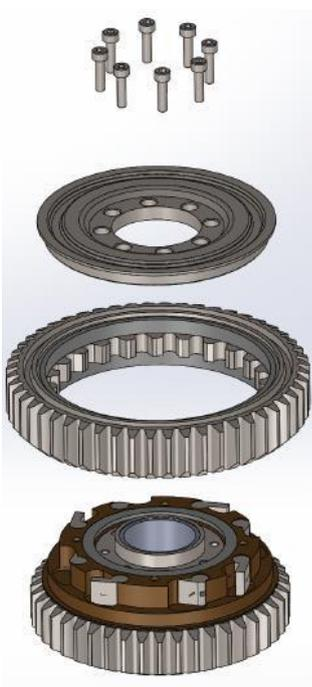
b. Turn the lower part of the gear set upside down and remove the 8 screws that hold it together. Lift off the closing plate and the freewheel gear to expose the bronze pawl carrier. Remove and clean the pawls and springs, checking the pawls and pawl pockets for wear. With normal use these pawl springs should be changed every two years or so.
