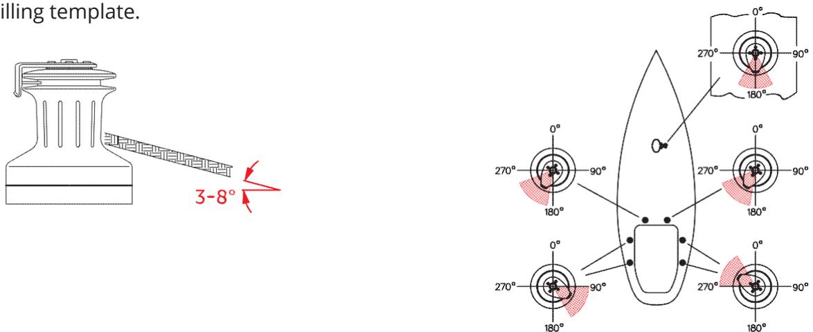
Note the drainage grooves on the underside of the winch base. If the mounting surface is not horizontal due to deck camber or other factors, plan the installation such that water may drain away from the winch base towards the lowest point in relation to the slope of the mounting surface.
