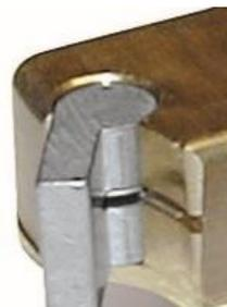
Correctly fitted in a pawl pocket
