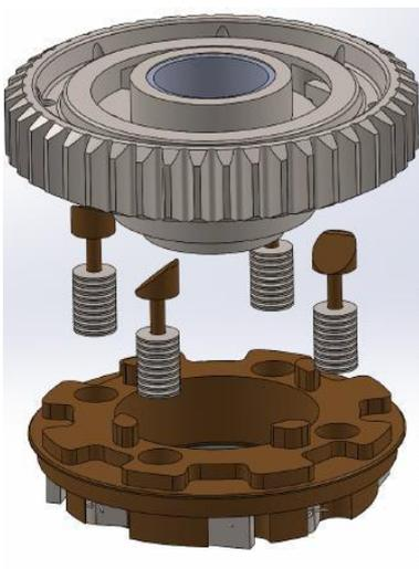
c. Turn over the pawl drive assembly and separate the drive gearwheel from the bronze pawl carrier to access the springs that control the gear shifting torque. Lift out and clean the springs; check the 4 angled sliders for wear.
