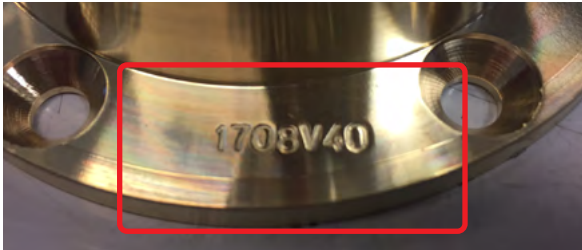
Winch production year and month [YY-MM] followed by version number engraved on base of centre stem.
