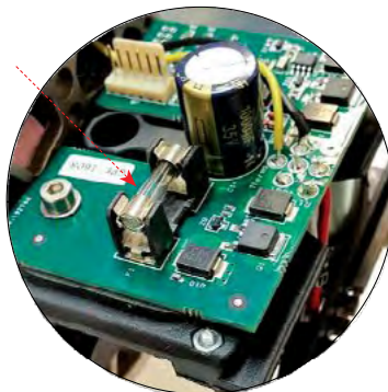
5A Glass Fuse PCB location
