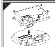
Install the Control Box properly with the included screws.
