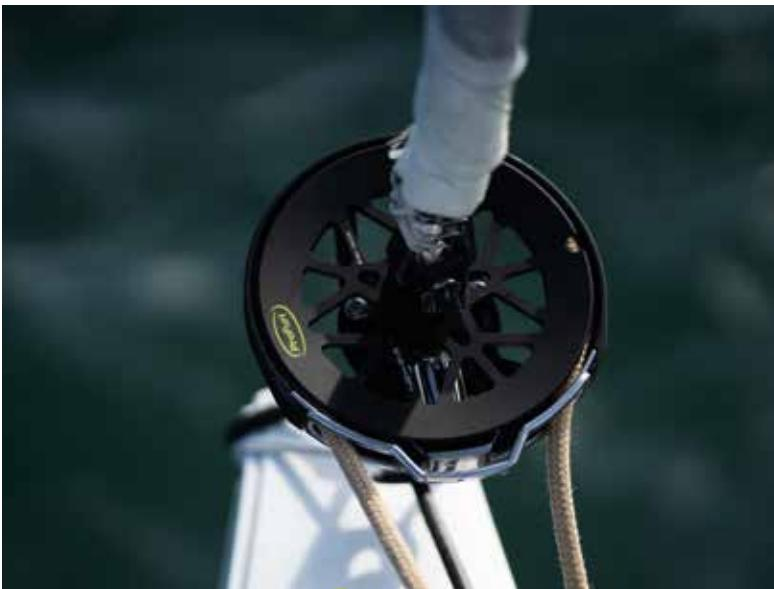
NEX furlers and manual furlers share the Profurl technology that has created the reputation of the brand: Profurl mechanisms are the only ones to use bearings made from very hard **100C6 carbon steel** which allow furling even under high loads (no crushing of the balls). The mechanism is mounted in a waterproof grease bath and is protected from external aggressions (salt, sand, etc.) and does not require any maintenance.
